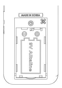
\*\*\* N.B : Make sure to insert the battery with the proper position of positive(+) and negative(-) as indicated.
